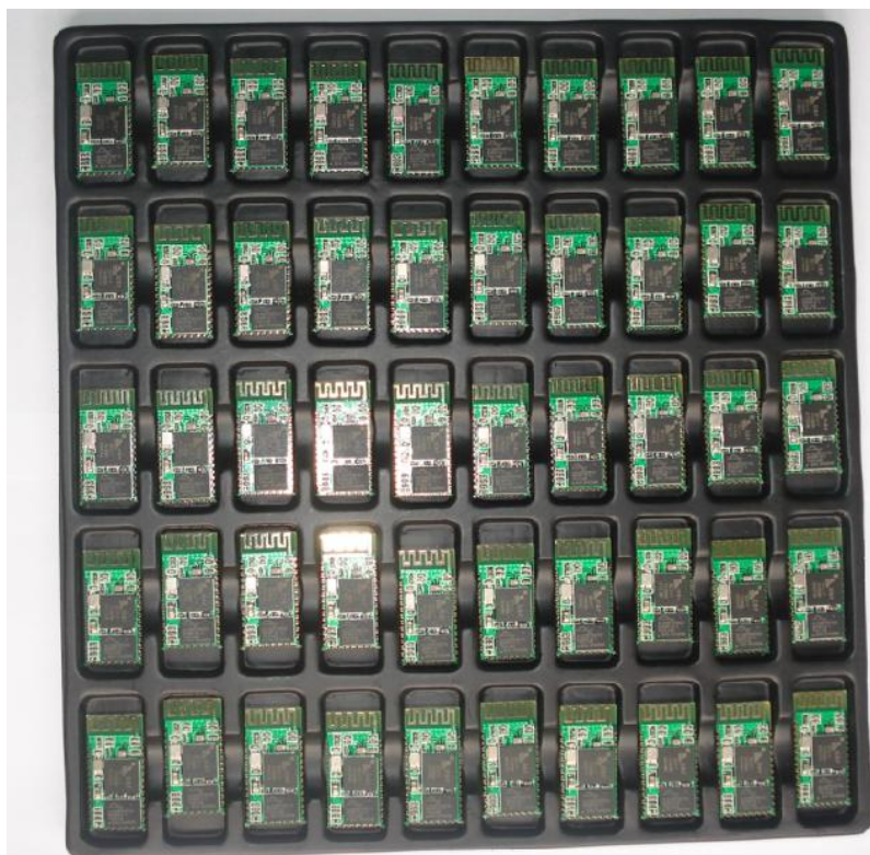
Figure 3 50 pieces chips in an anti-static blister package.
